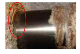
Inspect the seal wear. If any parts missing – can be a contamination issue.
