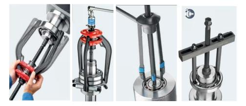
Use a suitable bearing puller
