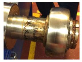
Using incorrect equipment and unnecessary force when removing the bearing can cause damage.
